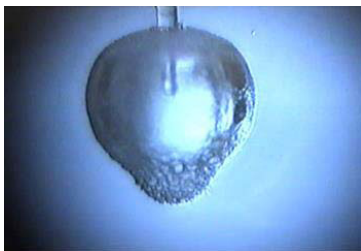
Holmium laser steam bubble at 2 Joules
